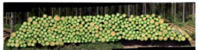
Fig. 3: Log count detection using full-surface end-face cross-caliper measurement
